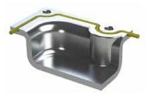
The minimum internal bend radius of a solid cord gasket is 1.5 x cross section of cord.
