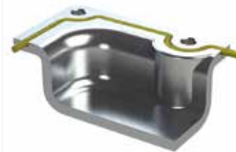
The minimum internal bend radius of a solid cord gasket is 1.5 x cross section of cord.
