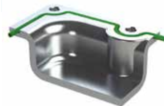
Minimum internal bend radius of a tube gasket where the id of the tube is no greater than 30% of the cross section is 2.5 x cross section of tube.
