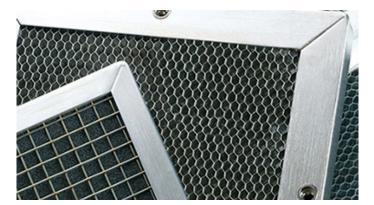
Honeycomb EMI vents. Honeycomb air ventilation panels consist of an aluminum honeycomb foil held in a rigid extruded aluminum mounting frame. The foil, formed and laminated into a series of honeycomb cells that are glued and perforated or laser welded at the join, ensures a conductive path at each join. Although the foil is conductive in all directions, to enhance EMI performance, two pieces of honeycomb polarized at 90° to each other are recommended.
